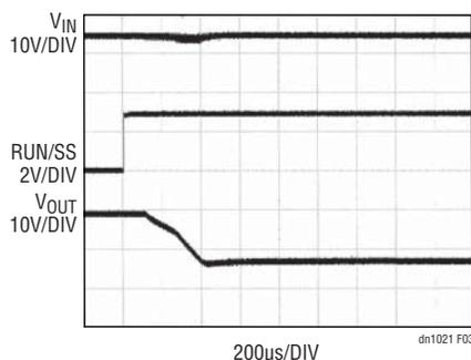
Figure 3. LTM8025 Start-Up Waveforms for -12V Output
