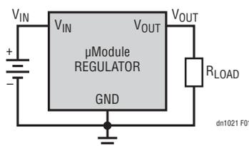
(a) Buck  $\mu$ Module Regulator Configured for Positive Output Voltages
