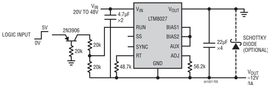
**Figure 5. LTM8027 with Run Level-Shift Circuitry for  $-12\text{V}$  Output**
