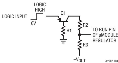
**Figure 4. Run Level-Shift Circuit for Negative Output Configuration**
