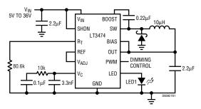
Figure 1. LT3474 High Voltage Buck LED Driver Regulates 1A
