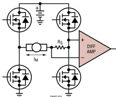
Figure 1. Classical Load Sensing Problematic with PWM
