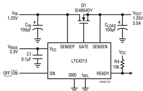
Figure 1. The LTC4213 in an Electronic Circuit Breaker Application
