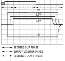
Figure 1. Sequencing Application Waveforms
