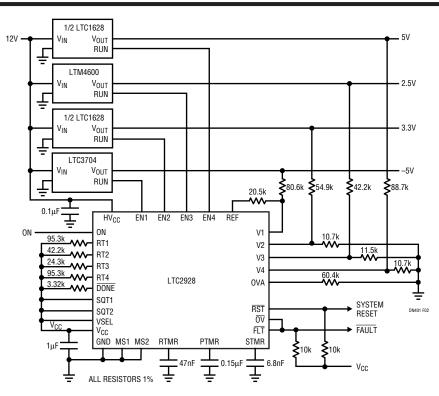
Figure 2. LTC2928 Application Schematic (component values calculated with the LTC2928 Configurator Tool)
