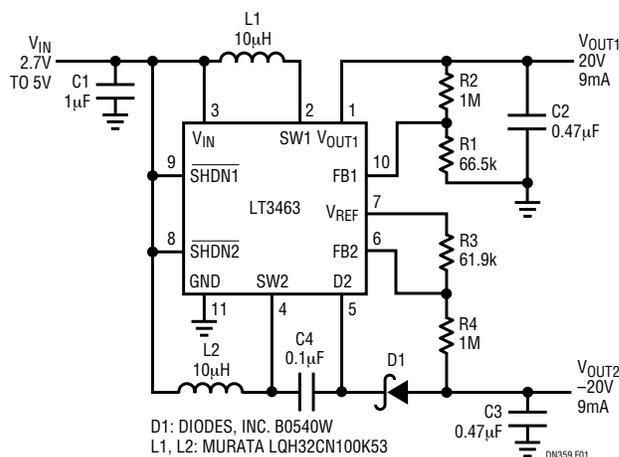
Figure 1. Dual Output  $\pm 20V$  Converter
