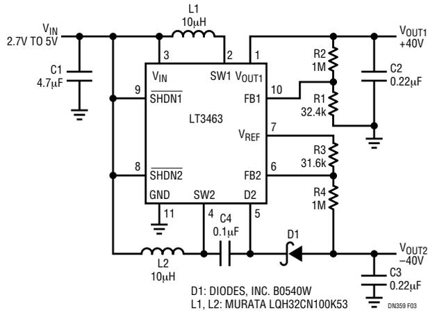
Figure 3. 2.7V to  $\pm 40V$  Dual Output Converter
