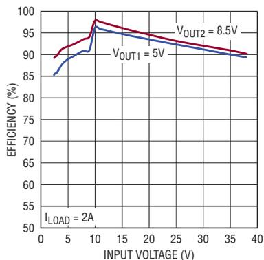
Figure 2. Efficiency vs input voltage for Figure 1.
