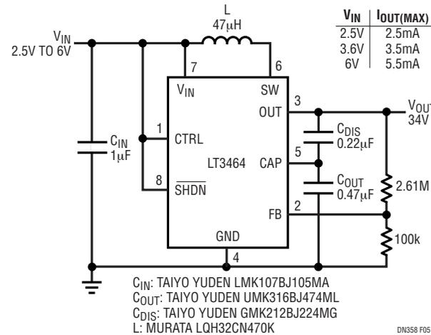
**Figure 5. 34V Bias Supply Using the LT3464**
