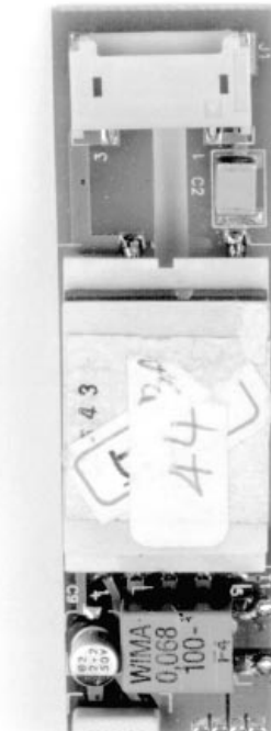
Figure G5. Transformer Output Terminals, Ballast Capacitor and Connector Are Isolated at End of Board. Slit Prevents Leakage
