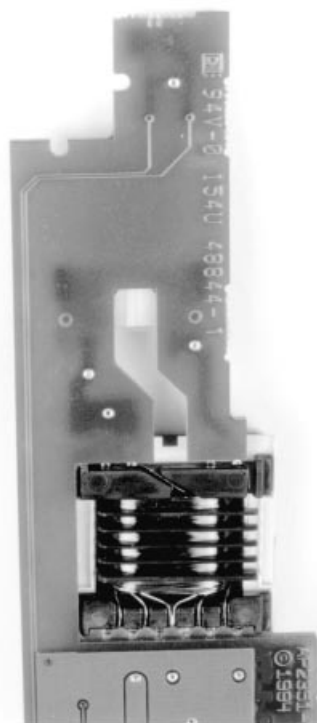
Figure G12. Bottom of G11 Shows Routed Area. Traces at Board Extreme Left Are Undesirable but Acceptable. Isolation Slit Between Traces and HV Points Would Be Preferable
