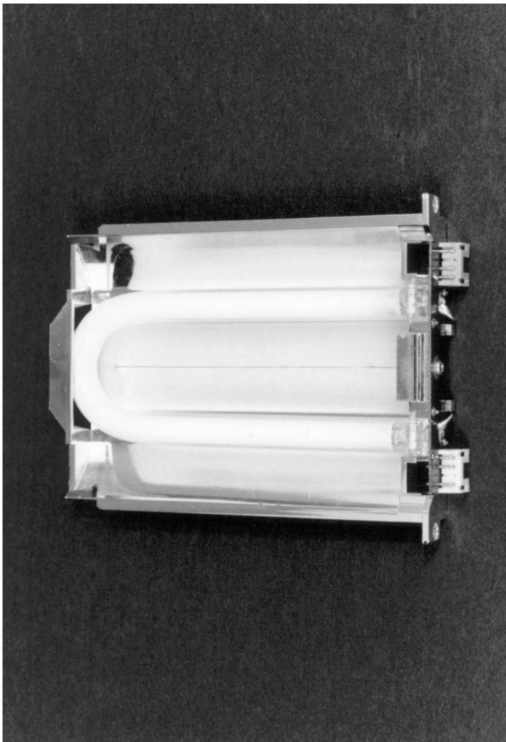
Figure 30. Grounded Metallic Optical Reflector in Automotive Lamp Introduces 18% Loss. Optical Gain over Nonmetallic Reflector May Justify Large Electrical Loss
