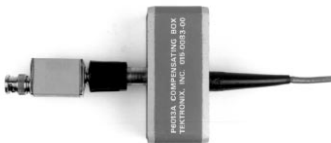
Figure C12. The Impedance Matching Box (Extreme Left) Mated to the High Voltage Probe. Note Direct Connection. No Cable Is Used
