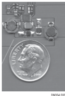
Figure 3. Typical Layout for a 5V Dual Phase Boost Converter
