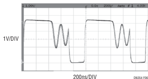
Figure 6. Switch Waveform for a 5V Single Phase Boost Converter in Discontinuous Mode
