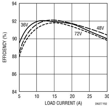
Figure 2. 36V to 72V<sub>IN</sub> to 3.3V<sub>OUT</sub> Efficiency
