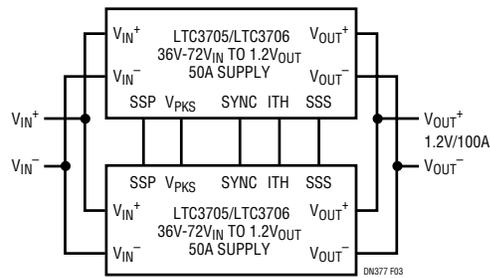
Figure 3. Paralleling Supplies for Higher Power Operation
