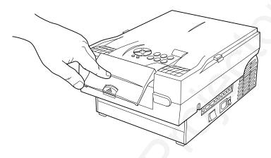
Figure i-12 Closing the lens
