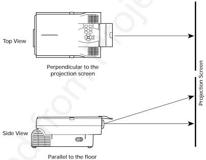
Figure 1-1 Positioning the projector
