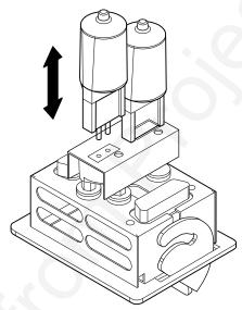
Figure 4-2 Removing a bulb
