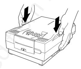
Figure 2-8 Releasing the projector top
