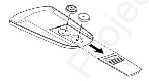
Figure 4-5 Installing batteries in the Cyclops Quick Remote
