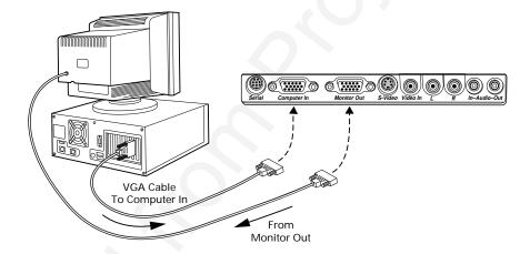
Figure 1-8 Connecting a PC
