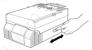
Figure 2-6 Correcting the keystoned image
