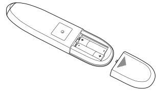
Figure 4-4 Installing batteries in the Cyclops Remote Control
