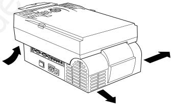
Figure 1-3 Allow for proper air flow
