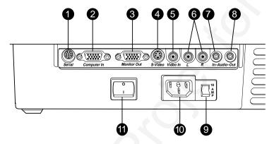
Figure i-6 The Connector Panel
