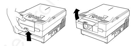
Figure i-4 Opening the lens
