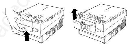
Figure 2-2 Opening the lens
