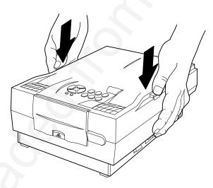
Figure i-13 Releasing the projector top
