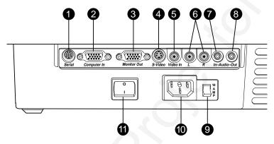
Figure 1-4 The Connector Panel
