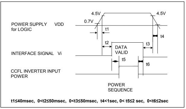
\* Set 0 Volt Vi(t) ≤ V<sub>DD</sub>(t) Here Vi(t), V<sub>DD</sub>(t) indicate the transitive state of Vi, V<sub>DD</sub> when power supply is turned ON or OFF
