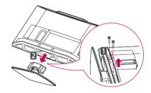
3 Push the supplied protection cover into the opening at the bottom of the TV until it locks in place.
