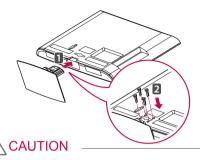
Tighten the screws firmly to prevent the TV from tilting forward. Do not over tighten.
