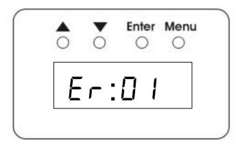
Error 01 is displayed for an overtemperature condition. Error 02 is displayed for an overvoltage condition.
