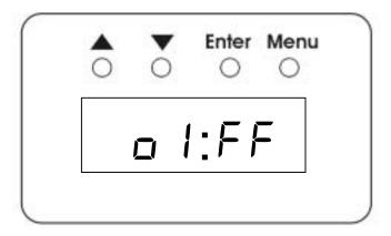
If a channel has been set to a fixed level in the Channel menu, the output status will reflect that level. In this case, the input for channel 1 could be zero, but there could be a non-zero output level.
