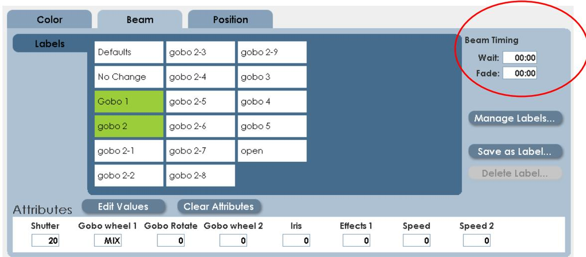
The Main record screen has the field for intensity fade times, and times that apply to all properties, such as Wait time.
