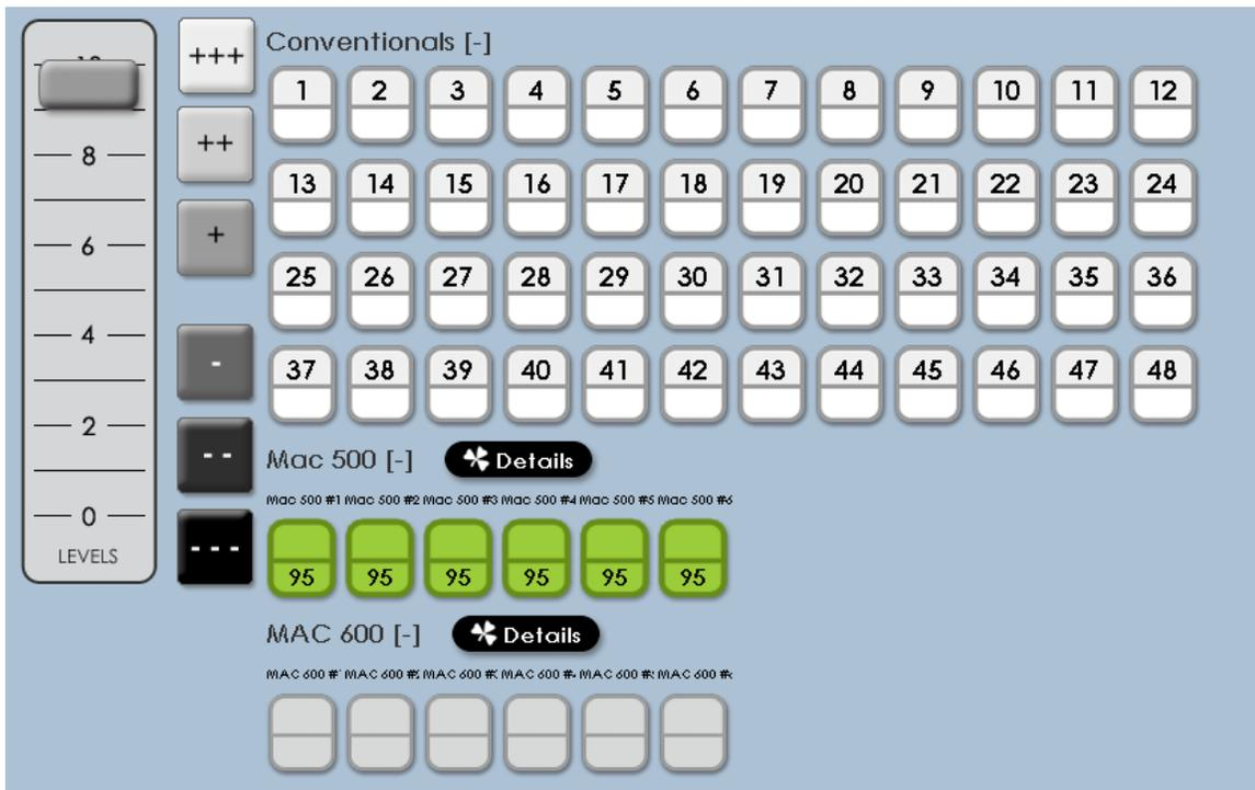
Clicking on the on-screen level controls, or using the 'level' key will adjust the intensity level of the intelligent fixture or LED. All other fixture parameters, such as color, position and beam will be unchanged from their current position.
