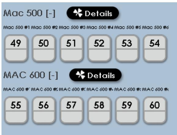
The fixtures in the illustration above were assigned with Intensity channels mapped to board channels. In the case shown, board channels 49 through 60 are used to control the intensity of the intelligent fixtures.
