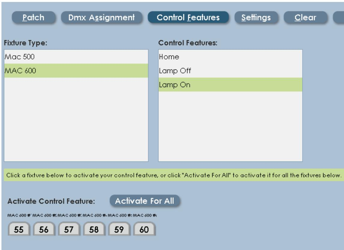
The image above shows Lamp ON selected. Click on individual fixtures to send Lamp On commands to those fixtures, or click 'Activate For All' to send Lamp On commands to all of the MAC600 fixtures.
