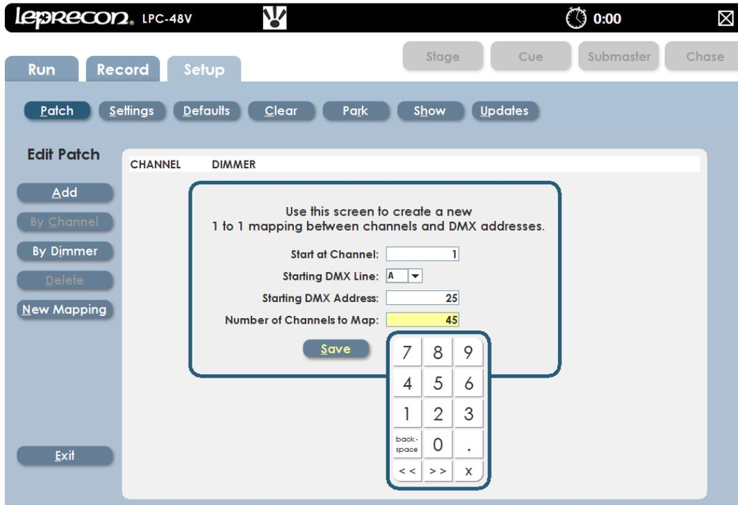
Figure 8: Patch Mapping Screen
