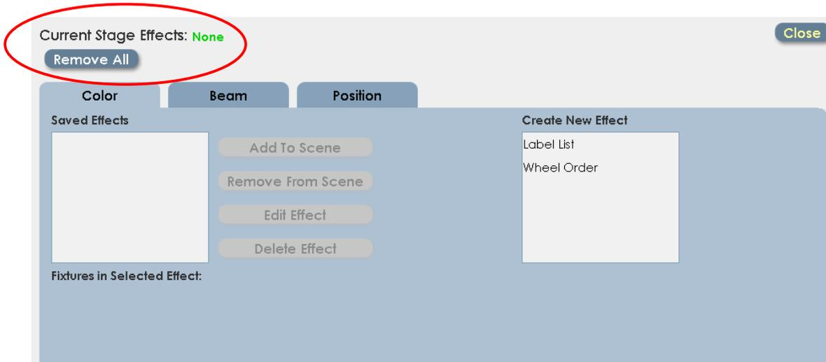
Note the top line of the screen – Current Stage Effects. This shows all currently running effects. If an Effect name is shown here, it will be included in any submaster or cue that is recorded.
