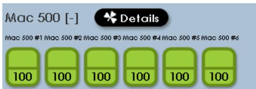
The small shamrock in the button indicates that the 'shamrock' key on the LPC front panel can be used for the same function. The 'shamrock' key is a quick way to toggle between the main display or record screen and the 'details' window.
