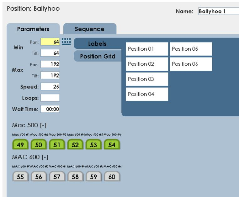
Clicking on a label will transfer the pan and tilt values for the label into the Min or Max data box.
