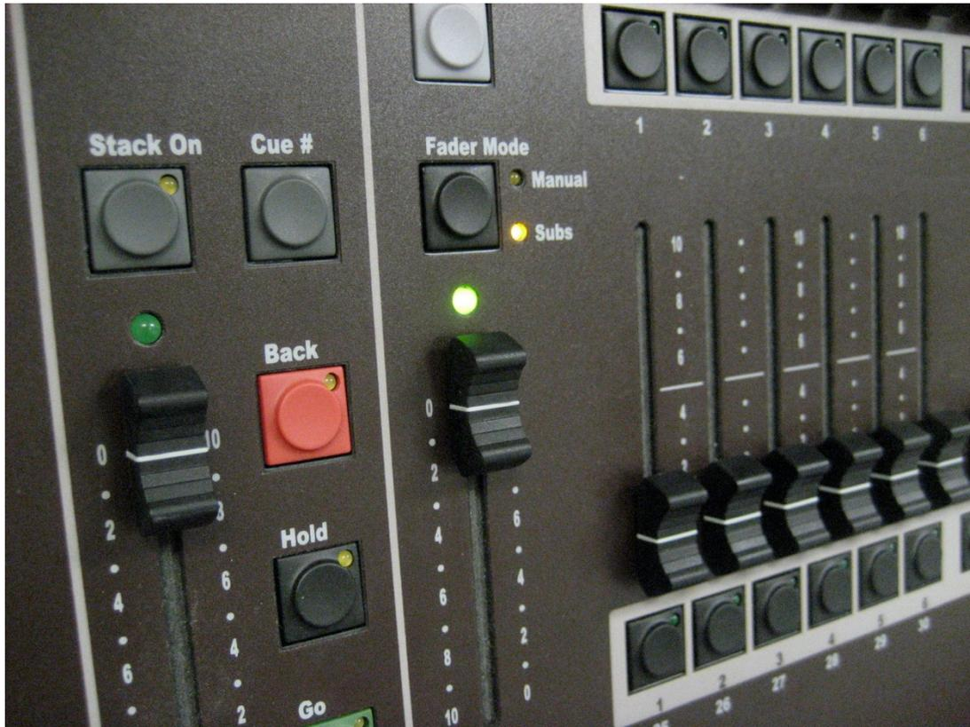
Figure 18: Fader Mode
