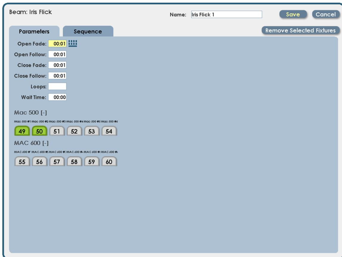
The properties for Iris Flick are simple, related to the time to open and close the iris, and the time between opening and closing the effect.
