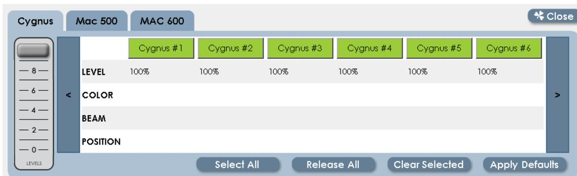
There is a tab at the top of the 'Details' screen for each type of fixture in the system. Clicking on one of the tabs will show the fixtures of that type.
