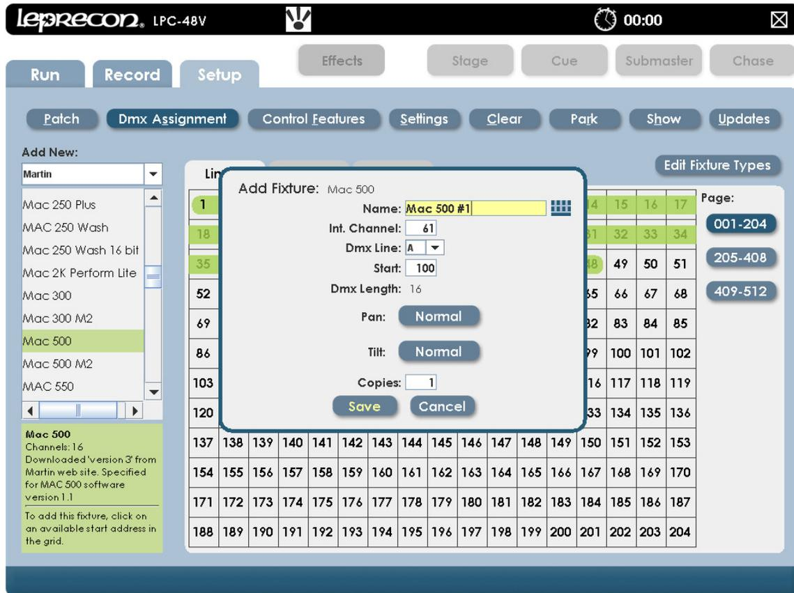
From the Setup Menu, choose DMX Assignment. Click the drop down box to show the list of available manufacturers, and pick the specific fixture from the manufacturer list.
