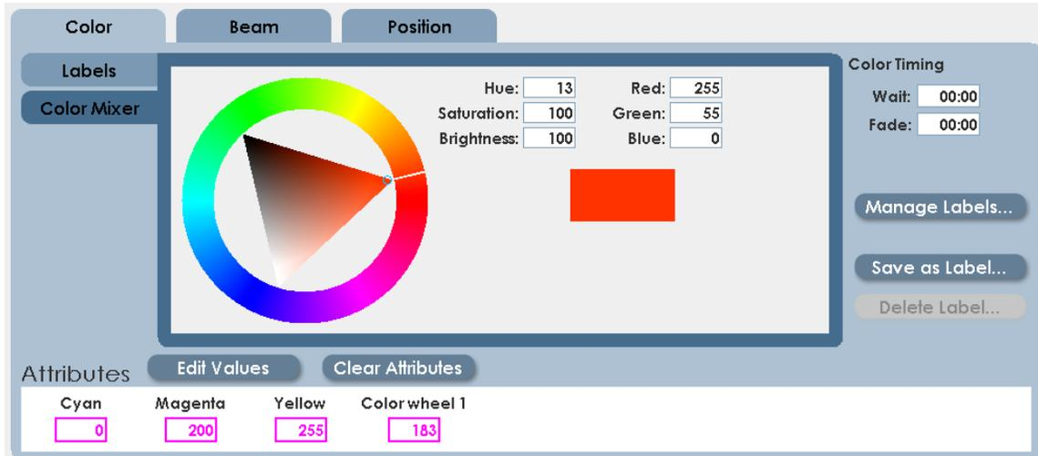
The Color mixer allows a range of color, saturation and brightness values for new labels.
