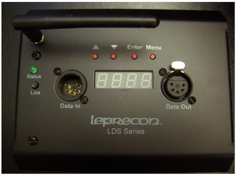
OFF - Dimmer is not linked to any transmitter. DMX cable input can be used.
