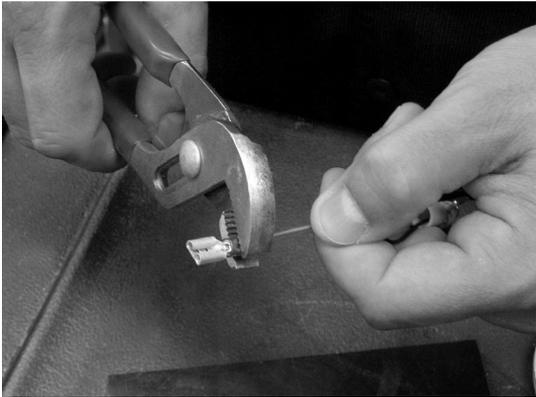
**Attach appropriate connectors to wire leads.**
