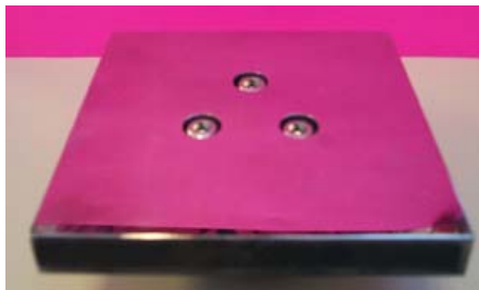
FIGURE 4. Upside Down View of Surface Plate with Recessed Screws
