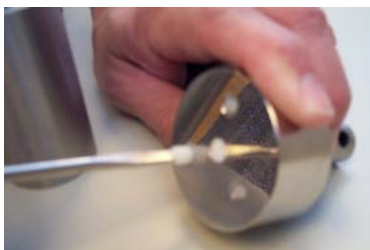
FIGURE 7. Tighten Slotted Nylon Screws
