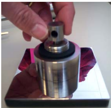
FIGURE 6. Inserting the Punch in the Intrinsic Apparatus
