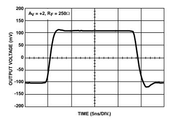
FIGURE 8. SMALL SIGNAL BIPOLAR PULSE RESPONSE
