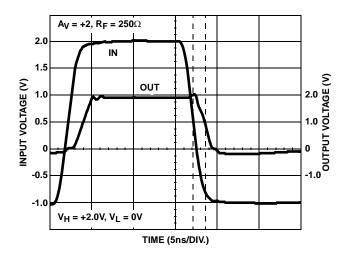
FIGURE 5. PULSE RESPONSE WITH LIMITING
