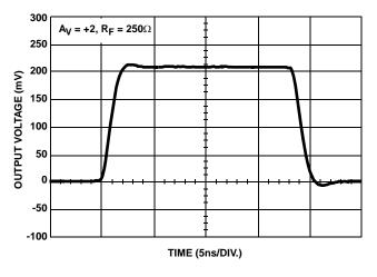
FIGURE 6. SMALL SIGNAL POSITIVE PULSE RESPONSE
