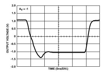
FIGURE 17. LARGE SIGNAL BIPOLAR PULSE RESPONSE
