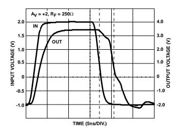
FIGURE 4. PULSE RESPONSE WITHOUT LIMITING
