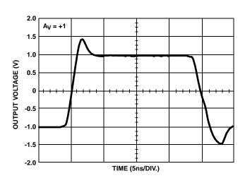
FIGURE 13. LARGE SIGNAL BIPOLAR PULSE RESPONSE
