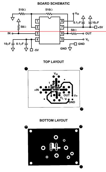
FIGURE 2. EVALUATION BOARD SCHEMATIC AND LAYOUT
