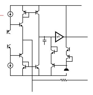
This current is mirrored onto the high impedance node (Z) by  $Q_{X3}$ - $Q_{X4}$ , where it is converted to a voltage and fed to the output via another unity gain buffer. If no limiting is utilized, the high impedance node may swing within the limits defined by  $Q_{P4}$  and  $Q_{N4}$ . Note that when the output reaches its quiescent value, the current flowing through -IN is reduced to only that small current (-I<sub>BIAS</sub>) required to keep the output at the final voltage.
