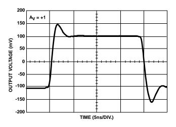
FIGURE 12. SMALL SIGNAL BIPOLAR PULSE RESPONSE
