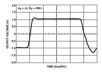
FIGURE 9. LARGE SIGNAL BIPOLAR PULSE RESPONSE
