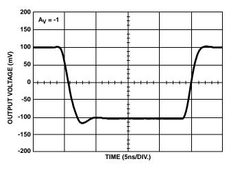
FIGURE 16. SMALL SIGNAL BIPOLAR PULSE RESPONSE
