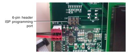
Connect the 6-pin ribbon cable connector to the ISP (In System Programming) port with the RED stripe toward the left-side as shown below.
