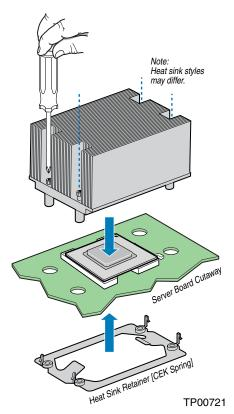
Figure 10. Installing the Heat Sink
