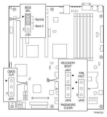
Figure 4. Configuration Jumper Location
