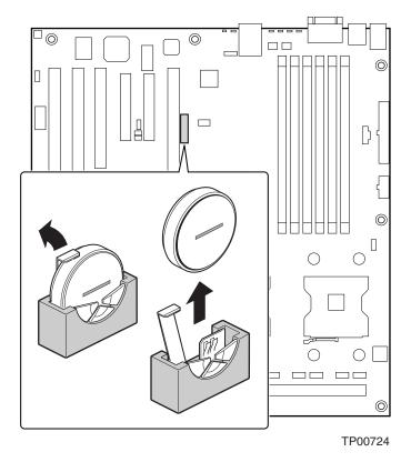
Figure 11. Replacing the Backup Battery
