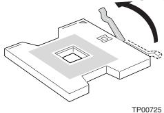
Figure 7. Opening Socket Lever
