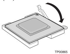
Figure 9. Closing Socket Lever
