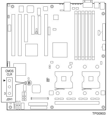
Figure 14. Clear CMOS Jumper
