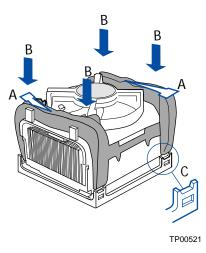
Figure 9. Attaching the Fan Heat Sink Clips to the Processor Socket
