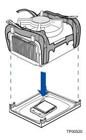
Figure 8. Attaching the Heat Sink to the Processor
