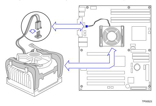
Figure 11. Connecting the Processor Fan Cable to the Processor Fan Connector
