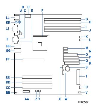
B: CPU Fan Header C: Sys Fan Header 3 D: +12 V CPU Power Connector E: Sys Fan Header 4 F: Processor Socket G: DIMM 2B Socket H: DIMM 2A Socket I: DIMM 1B Socket J: DIMM 1A Socket
