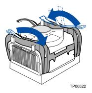
Figure 10. Attaching the Fan Heat Sink Clips to the Processor Socket
