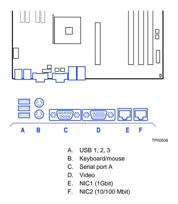
**Figure 5. Back Panel Connectors**
