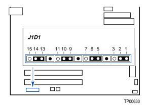
Figure 4. Configuration Jumper Location
