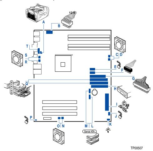
Figure 3. Making Connections to the Server Board
