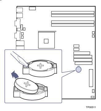
Figure 12. Replacing the Battery
