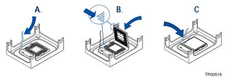
Figure 7. Installing the Processor in the Processor Socket
