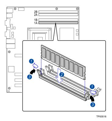
Figure 6. Installing Memory
