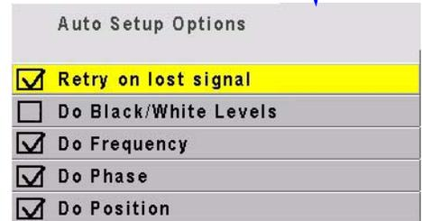
**Do Frequency** and **Do Phase** automatically adjust the electronics module to the frequency and phase of the selected picture.
