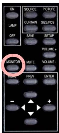
Press MONITOR twice to open the RS-232 Serial Port Status menu. Push three times to open the RS-485 Serial Port Status.
