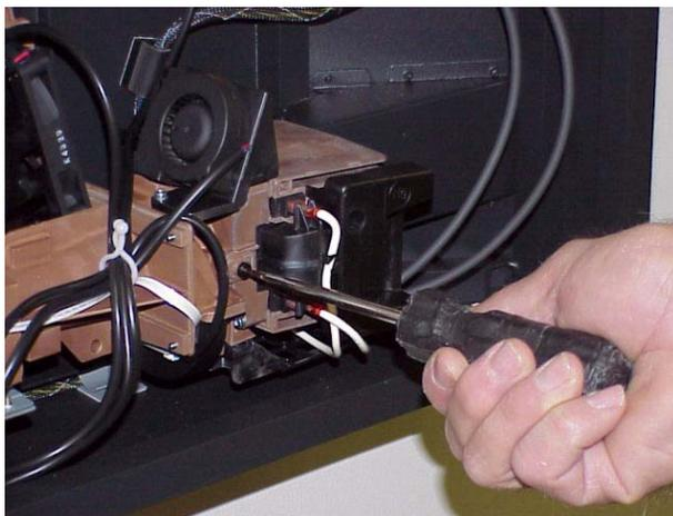
4. Use screwdriver to loosen the captive screw holding the lamp in place.
