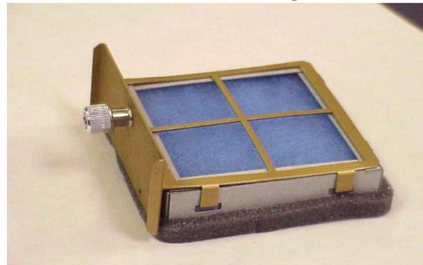
4. This is the TD61 filter in its holder. Remove the foam filter from the filter holder.
