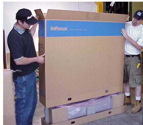
4. Slide the box sleeve up and off of the TD61
