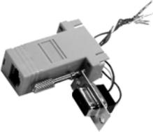
This little 9-pin to RJ45 adapter is available unwired from many computer or electronic stores. Get one with a female 9-pin connector.
