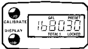
The “field” calibration curve(s) may be set by the user, and can be changed or modified at any time using the calibration procedure described below in the CALIBRATION section. Totals or flowrate derived from the field calibration are visible when the field calibration setting is selected (“CAL B” or “CAL C” will be visible).
