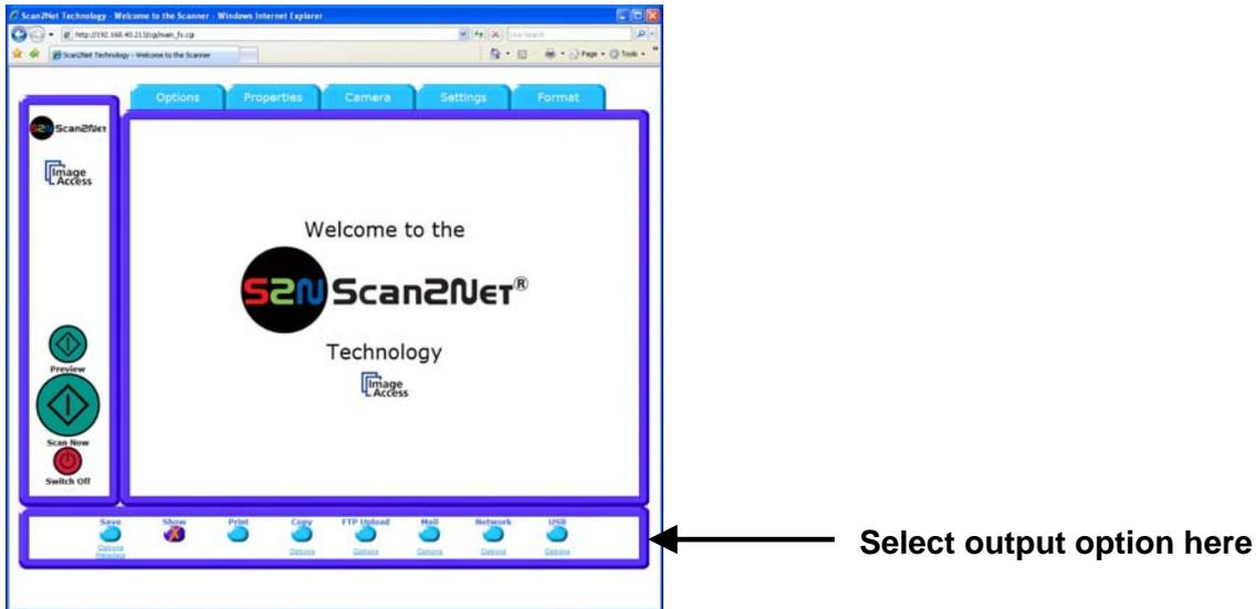
There are eight output options available on a Scan2Net scanner, selectable at the bottom part of the main window.
