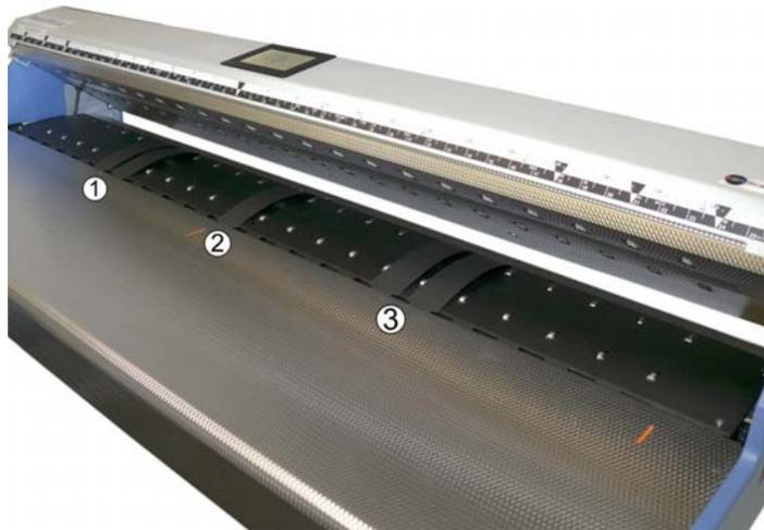
**Picture 8: Position of paper transport wings**
