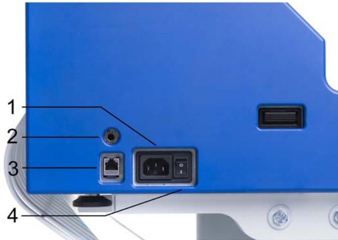
**Picture 3: Connectors at WideTEK 42/WideTEK 48**
