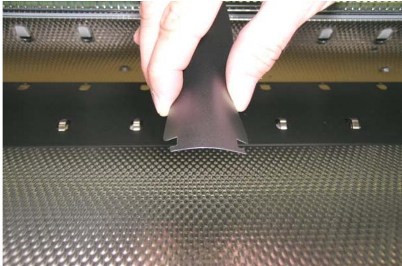
**Picture 6: Bending the paper transport wing**
