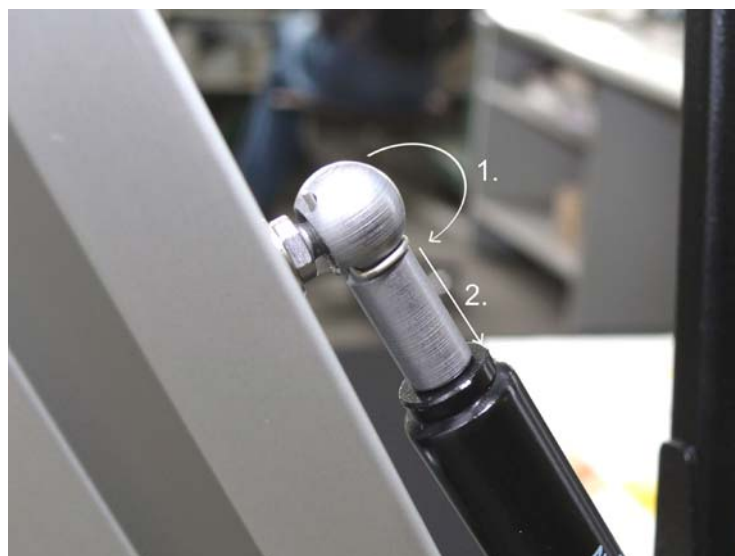
Picture 35: Removing the locking spring
