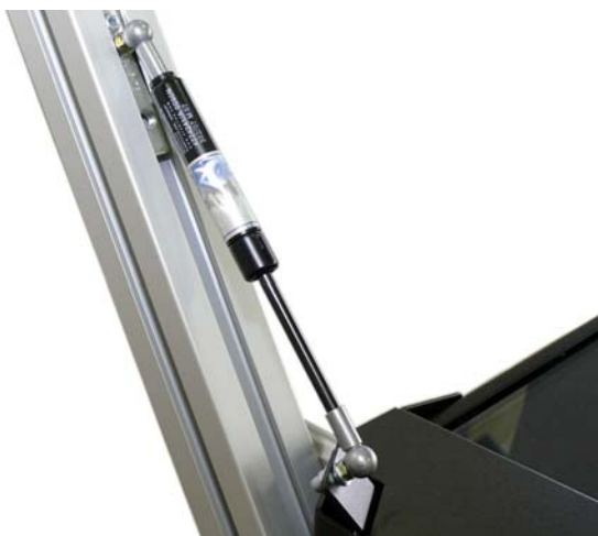
Picture 39: Gas spring completely mounted
