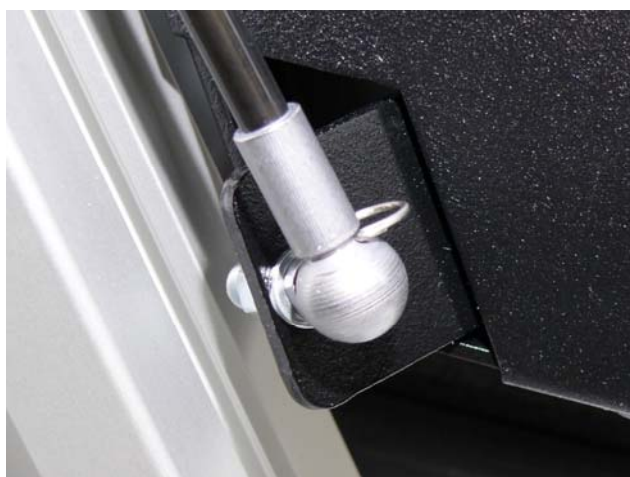
Picture 37: Locking spring inserted
