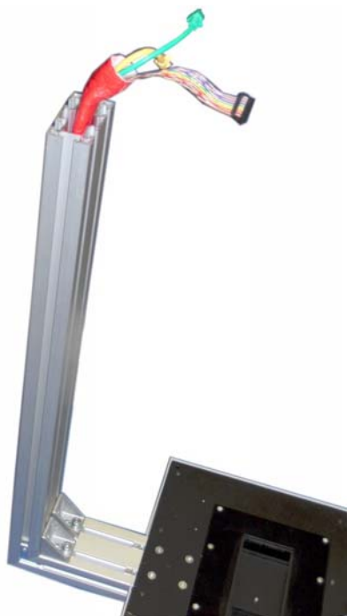
Picture 11: Camera neck assembled at camera head
