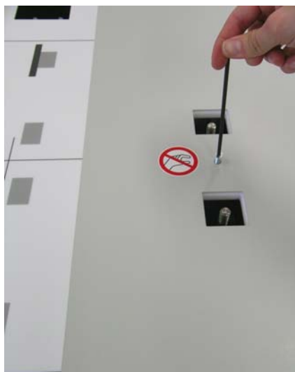
Picture 17: Removing the countersunk socket screw
