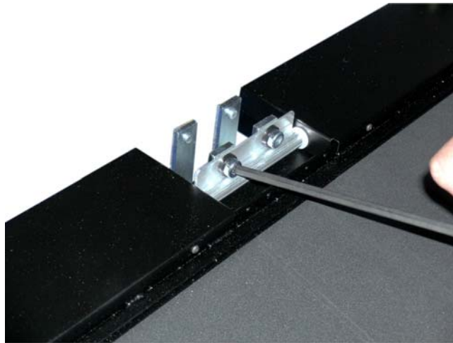
Picture 16: Removing the transport screws
