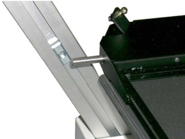
Picture 32: T-slot nut in corresponding position
