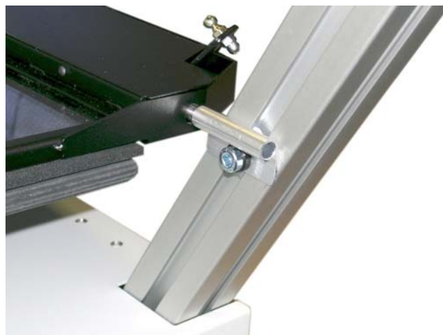
Picture 33: Hinge mounted at right lamp
