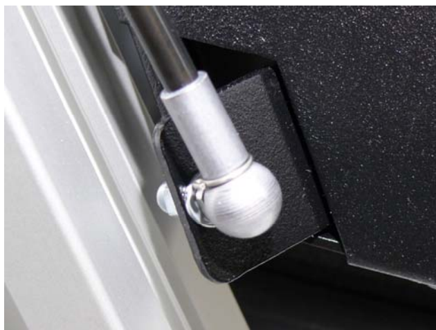
Picture 38: Locking spring locked
