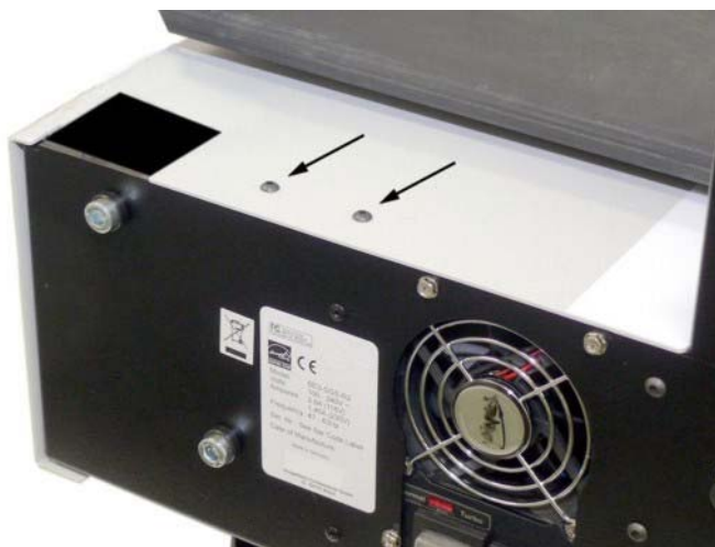
Picture 18: Remove marked screws
