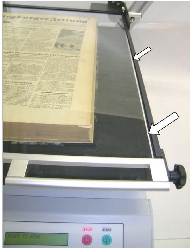
**Picture 8: Horizontal alignment check**
