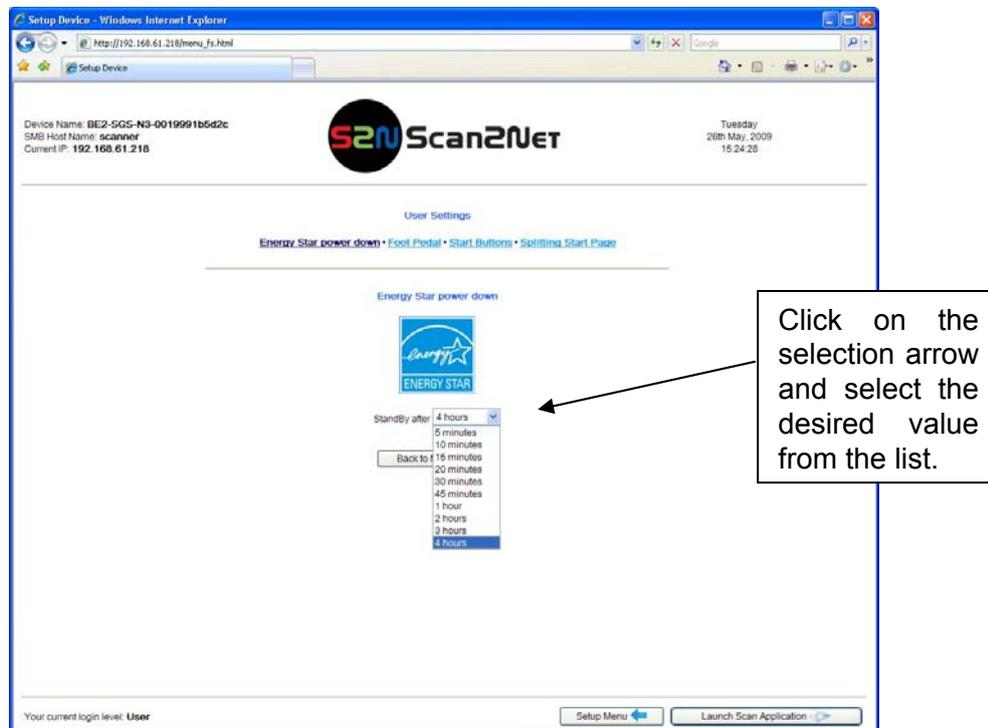
In stand-by mode it consumes only 5W of power. The Energy Star guidelines require the default time until the device goes into standby to be 15 minutes. Select the desired time from the list.
