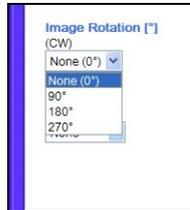
The **Image Rotation** can be any degree of rotation out of 90°, 180°, 270° or none. The rotation angle is defined in clockwise direction.
