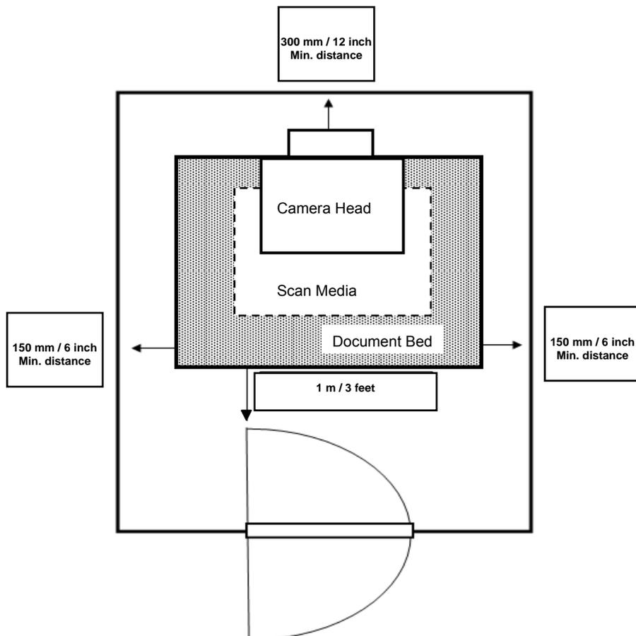
Do not operate the scanner in an area that has poor air circulation, and/or that is non-ventilated.
