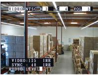
Press the MODE button repeatedly to change the the Video Tester screen indicated by "VIDEO" in the upperleft corner of the screen.
