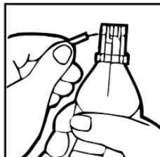
**(GB)** Place wire in jaws in proper blade hole.
