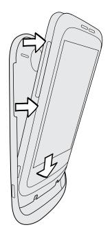
2. Press the sides and top part of the back cover towards the phone to lock the cover in place. You'll hear a click when the back cover is locked in place.
