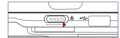
On the right side of your Mobile Computer, slide the Power/Hold switch to the right for 1 to 2 seconds to turn on the power.
