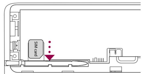
The USIM/SIM card slot is inside the battery compartment.
