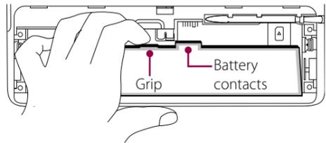
**Note** Slide the battery latches outward to release the battery. Remove the battery by lifting it up from the protruding grip that is located beside the battery contacts.
