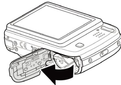
3. Insert the batteries into the compartment with correct orientation as illustrated.
