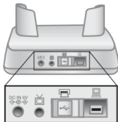
There is a sliding door over the computer and printer connectors that prevents you from selecting both connectors at the same time (the camera dock is not a USB hub).
