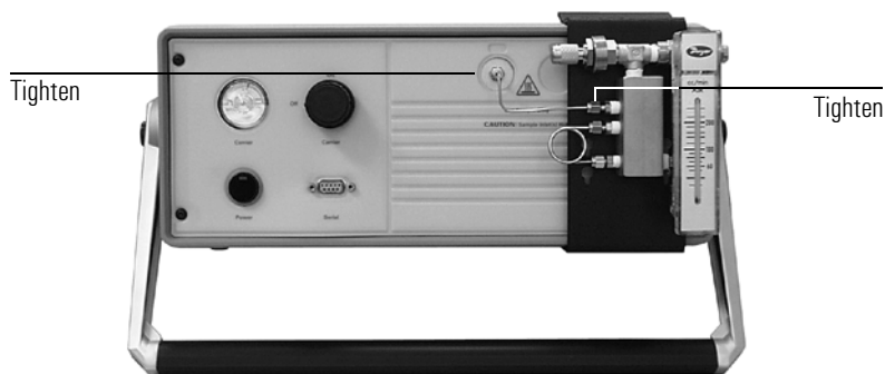
Figure 6. Tighten the fittings
