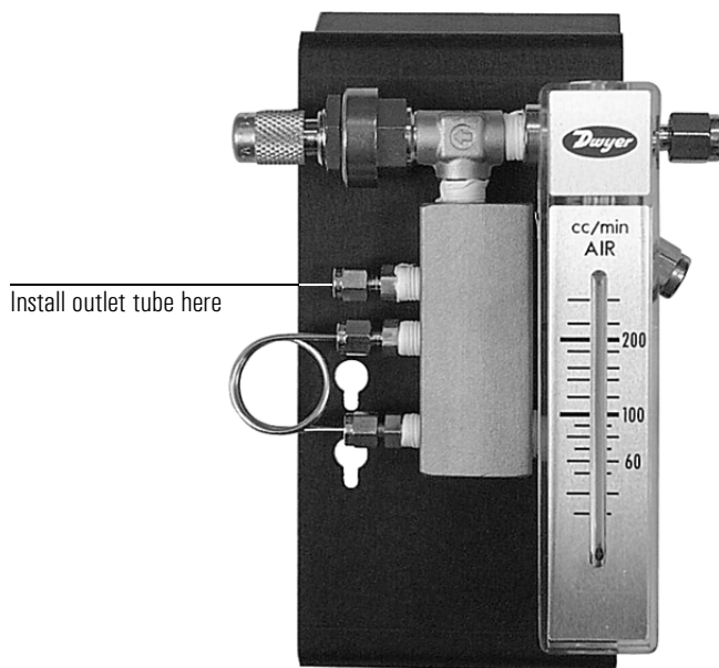
Figure 3. Installing the sample outlet tube
