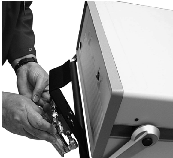
Figure 4. Installing the bracket onto the GC
