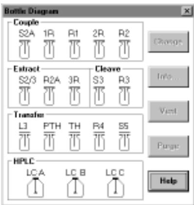
The Routine 4.0 sequencer methods require the bottle configuration shown. The reagents and solvents are purchased from Hewlett-Packard. These methods produce less than 1mL/cycle of liquid waste.
