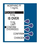
All soft limit overrides made during programming are indicated on the INFUSION SCREEN with an appropriate upper or lower limit arrow. See Important Symbols on page 6-11 for details.
