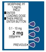
13 The Deliver Loading Dose Now Screen allows the option of delivering the loading dose now or after the programming is complete.
