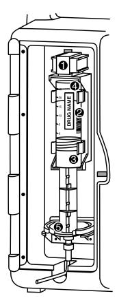
Squeeze Cradle Release Mechanism together at the top of the holder and move to the uppermost position.
