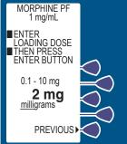
12 The Deliver Loading Dose Now Screen allows the option of delivering the loading dose now or after the programming is complete.
