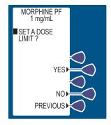
If Hospira MedNet™ Software is enabled and a upper hard or soft limit has been assigned for that CCA and drug, then a Dose Limit entry is required, and this screen will not be displayed.
