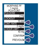
Press to begin therapy. Approximately 10 seconds after door is locked and is pressed, the DOOR LOCKED MESSAGE disappears.
