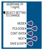
4 Enter the desired PCA dose using the numeric keypad. (The value range is displayed on the screen.) If the value is entered incorrectly, press to change value.
