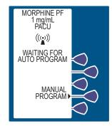
This symbol indicates that the PCA Infuser is connected to the wireless network. It does not indicate if data is currently being sent or received. The Waiting for Autoprogram Message will display on the screen.
