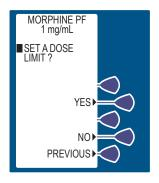
2 Enter the 4 HOUR DOSE LIMIT value using the numeric keypad.
