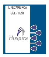
This screen is followed by another screen displaying self-test information that includes the following: time, date, drug library, software version and copyright data. During the self-test, the infuser reads the bar code label.
