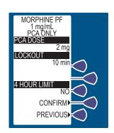
Approximately 10 seconds after the door is locked, the DOOR LOCKED Message disappears. After delivering the PCA dose, the PCA LOCKOUT Message appears indicating the PCA Infuser is locked out.
