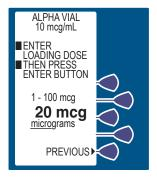
17 The Deliver Loading Dose Now Screen allows the option of delivering the loading dose now or after the programming is complete.
