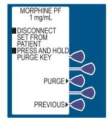
**NOTE:** Purging is recommended to remove system slack when a new vial is inserted. The maximum volume delivered during a purge is 3 mL.
