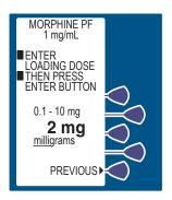
The next screen offers the options of infusing the loading dose now or later (after programming is complete). If Deliver Loading Dose Now? is desired, press the Yes> Softkey to infuse the programmed Loading Dose.
