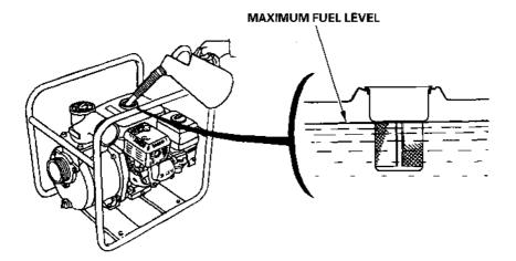
Refuel in a well-ventilated area before starting the engine. If the engine has been running, allow it to cool. Refuel carefully to avoid spilling fuel. Do not fill the fuel tank above the fuel strainer shoulder. After refueling, tighten the fuel tank cap securely.
