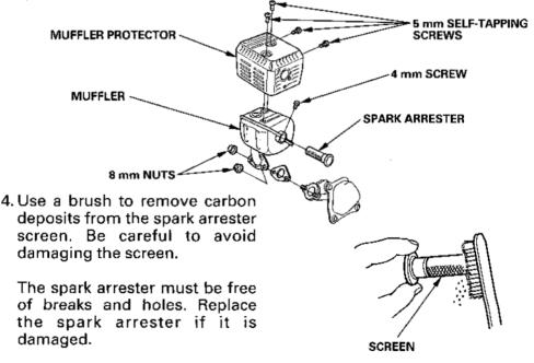
5. Install the spark arrester and muffler protector in the reverse order of disassembly.
