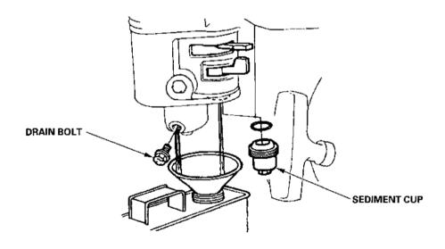
3. After all the fuel has drained into the container, reinstall the drain bolt and sediment cup. Tighten them securely.
