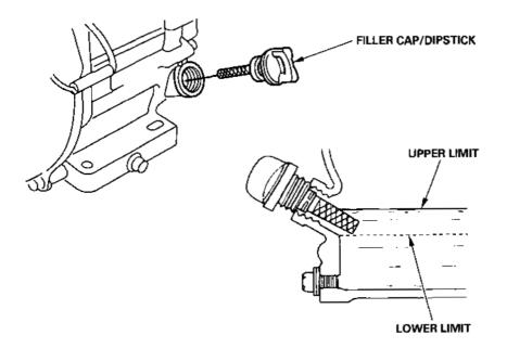
The Oil Alert<sup>®</sup> system will automatically stop the engine before the oil level falls below safe limits. However, to avoid the inconvenience of an unexpected shutdown, check the oil level regularly.
