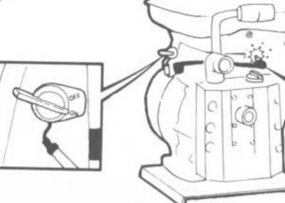
Pull the starter while touching the spark plug against the engine. If a spark in visible, reinstall the spark plug and try to start the engine. If there is no spark, clean or replace the spark plug.
