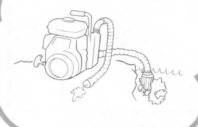
B-3. Are the hoses clamps tightened? Are the packing damaged?
