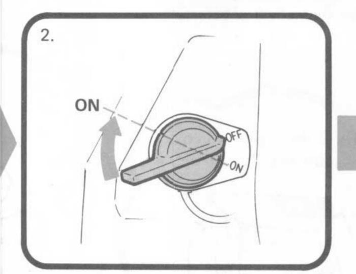
Turn the engine switch ON.
