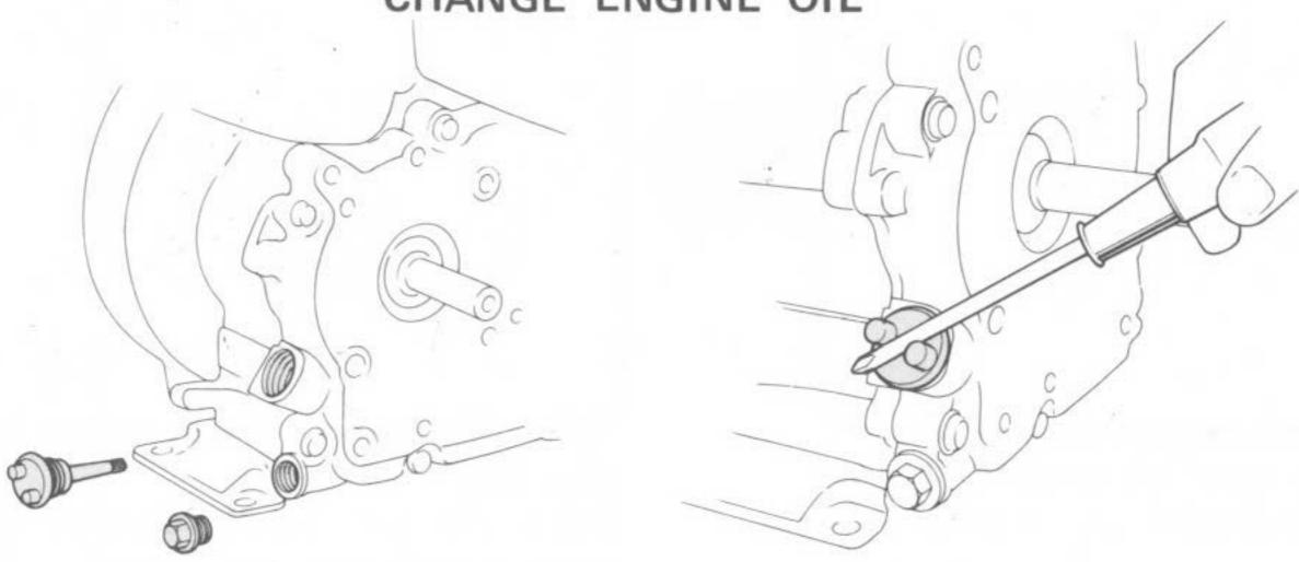
Use a screwdriver shaft to loosen or tighten oil filler cap.
