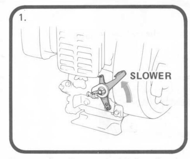
Loosen the wing nut and fully raise the throttle lever.
