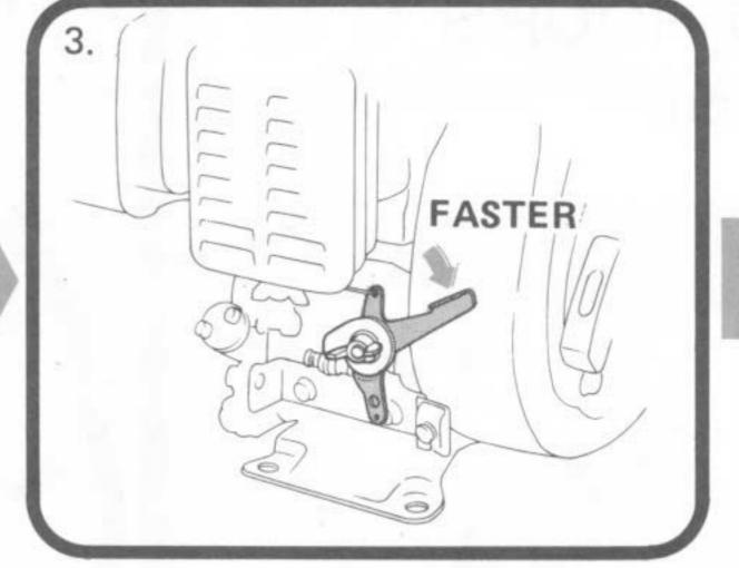
Loosen the wing nut, move the throttle lever down slightly and re-tighten the wing nut.
