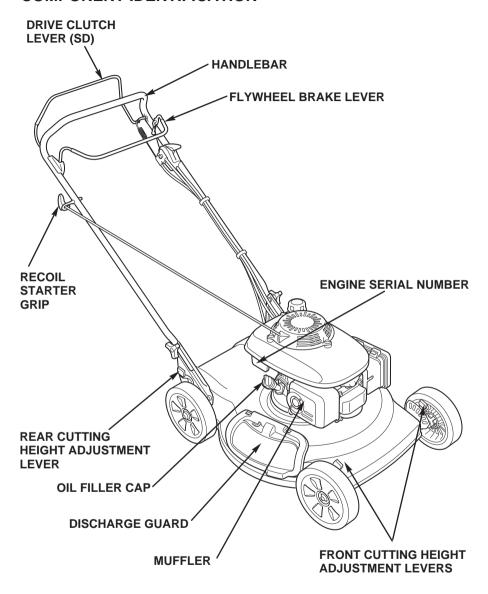
HRS216PD: Manually propelled (push) HRS216SD: Self-propelled, single speed
