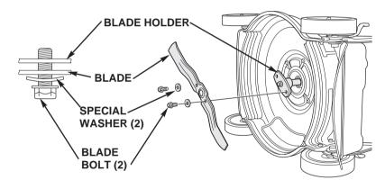
The blade bolts and washers are specially designed; when replacing them, use only genuine Honda parts. Tighten the bolts with a torque wrench. Use a wooden block to stop the blade from turning.
