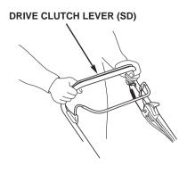
Operate the drive clutch lever with a quick and complete motion, so the drive clutch is either fully engaged or released. Hold the drive clutch lever against the handlebar during self-propelled mowing. This will help to extend the service life of the clutch mechanism.
