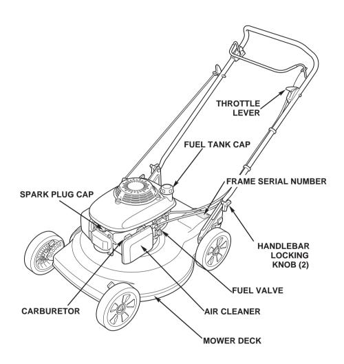
Record the frame and engine serial numbers in the space below. You will need these serial numbers when ordering parts and when making technical or warranty inquiries (see page ).
