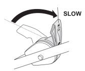
2. Release the drive clutch lever (SD).
