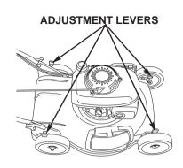
To adjust cutting height, pull each adjustment lever toward the wheel, and move it into another notch.
