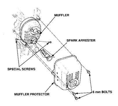
3. Use a brush to remove carbon deposits from the spark arrester screen. Be careful to avoid damaging the screen.
