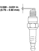
If reinstalling a used spark plug, tighten 1/8 - 1/4 turn after the spark plug seats.
