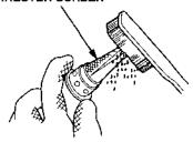
Install the spark arrester and muffler protector, in the reverse order of disassembly.
