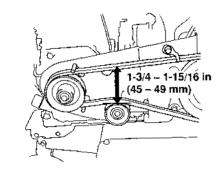
To adjust, loosen the four engine mounting bolts and the three inner belt cover tightening bolts and move the engine forward or backward to get proper tension on the belt.
