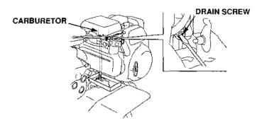
After all the fuel has drained into the container, tighten the drain screw securely.
