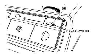
5. Flip the remote control engine switch knob up to ON.
