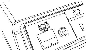
5. After the engine starts, let the engine switch return to ON.
