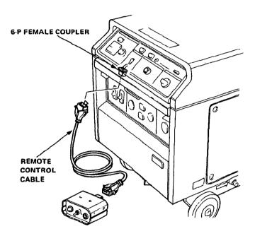
7. Connect the remote control 6-P male coupler to the switch box.
