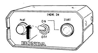
6. Depress the starter button until the pilot lamp is on.
