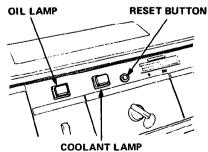
CAUTION: If engine idle speed is set too low, the protection circuit cannot be activated while idling. The correct idle speed is 2200 ± 200 rpm.
