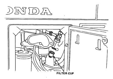
d. Drain the carburetor by loosening the drain screw. Drain the gasoline into a suitable container.
