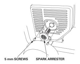
2. Use a brush to remove carbon deposits from the spark arrester screen.
