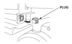
2. Connect the remote control cable to the back of the control panel and remote control box.
