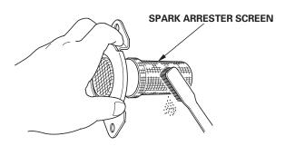
3. Install the spark arrester in the reverse order of removal.
