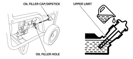
The Oil Alert system will automatically stop the engine before the oil level falls below safe limits. However, to avoid the inconvenience of an unexpected shutdown, check the oil level regularly.
