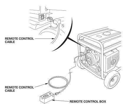
• When the remote control is not being used, replace it with the plug on the connector.
