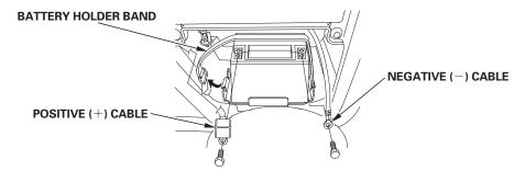
4. Remove the battery from the battery tray.
