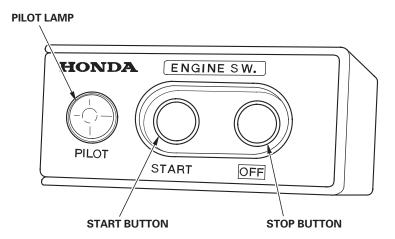
Starting the engine with remote control
