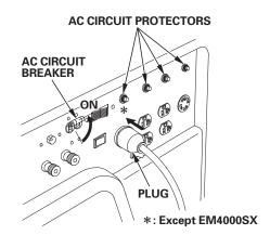
Do not exceed the current limit specified for any one receptacle. If an overloaded circuit causes the AC circuit breaker or AC circuit protector to switch OFF, reduce the electrical load on the circuit, wait a few minutes and then reset the AC circuit breaker or AC circuit protector.
