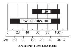
SAE 10W-30 is recommended for general, all-temperature use. Other viscosities shown in the chart may be used when the average temperature in your area is within the indicated range.
