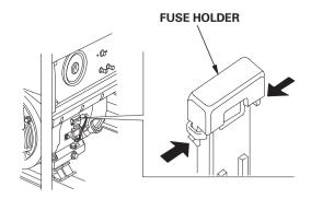
If frequent fuse failure occurs, determine the cause and correct the problem before attempting to operate the generator further.
