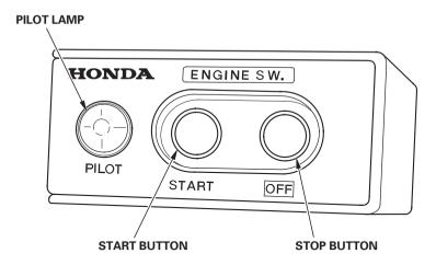
Starting the engine with remote control
