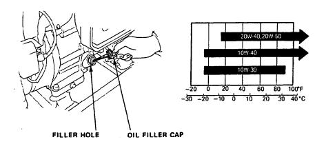
NOTE: When the oil runs lower than the specified level during operation, the oil alert switch automatically turns off to protect the engine from overheating.
