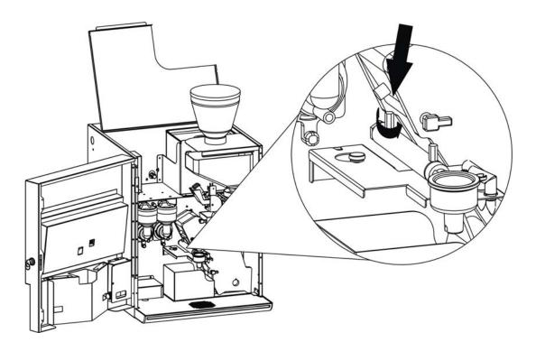
Pull out the entire steam tube. Unscrew completely the second brass Knob and disassemble the steam tube as showed in the following picture. Paying attention to not lose the components wash it in hot water, using a detergent. Dry thoroughly.
