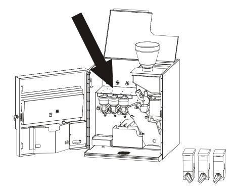
• Insert the switch locker on the front door. Put an empty cup or any other container under the drink nozzles and push the red button inside the door to start the cleaning cycle of the 4 drinks pipes and of the whippers.
