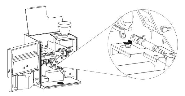
To remove the coffee group, simply turn each of the four levers to the 12:00 position, take off the hose on the front of the coffee group, and pull it straight out.
