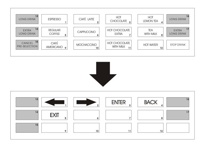
Buttons 1 and 2 are used to move forward or backward throw the various programming functions. These buttons are also used to decrease and to increase the various product doses and water amounts.
