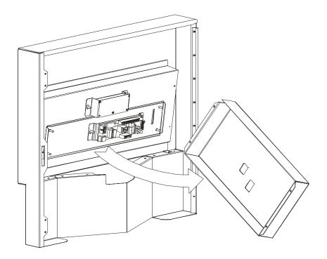
Unscrew the four nuts that hold the computer board bracket and lift it up as showed:
