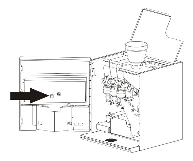
If during this process the message **CAUTION Flow Meter K.O.** appears, press for 1 second the red button to reset the machine.
