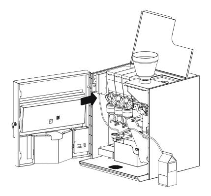
Then pull out the milk frothier holding in the same time the milk bottle with your right hand, and bring everything close to the sink in order to avoid spilling of milk.
