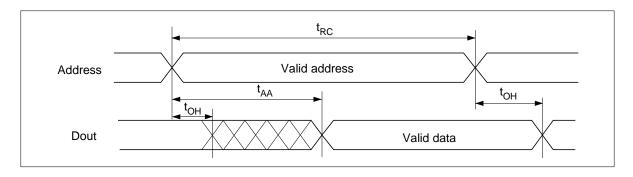
Read Timing Waveform (3)  $(\overline{WE}=V_{IH},\,\overline{OE}=V_{IL})^{*3}$
