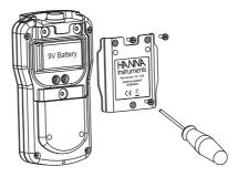
Make sure the battery contacts are tight and secure before replacing the cover.
