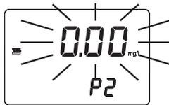
**Under Range:** A blinking "0.00" indicates that the sample absorbs less light than the zero reference. Check the procedure and make sure you use the same cuvette for reference (zero) and measurement.
